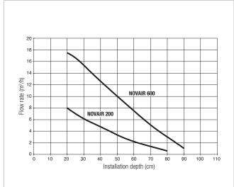
$\label{eq:thm:product} The performance curves are based on kinematic viscosity values = 1 \ mm^2/s \ and \ density \ equal \ to \ 1000 \ kg/m^3. \ Curve \ tolerance \ according \ to \ 150 \ 9906.$
