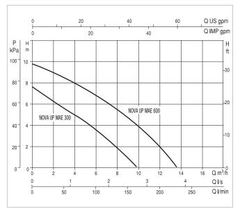
$\label{eq:thm:product} The performance curves are based on kinematic viscosity values = 1 \ mm^2/s \ and \ density \ equal \ to \ 1000 \ kg/m^3. Curve \ tolerance \ according \ to \ ISO \ 9906.$
